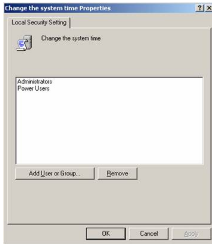
Figure 3: The list shows that only Administrators and Power Users are allowed to change the system time.
