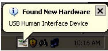
*Figure 2: "Found New Hardware" message indicates the USB 1024ls has been detected.*
