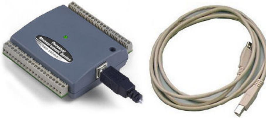
*Figure 1: The USB 1024ls and supplied USB cable are shown.*
