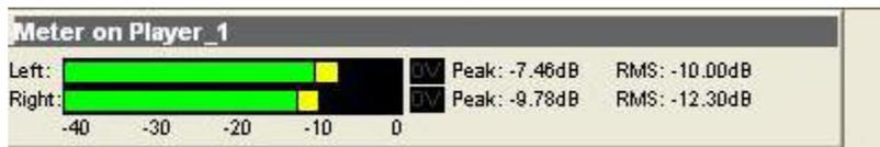
A stereo peak meter display. The RMS is the green bar and the peak is the yellow bar.
