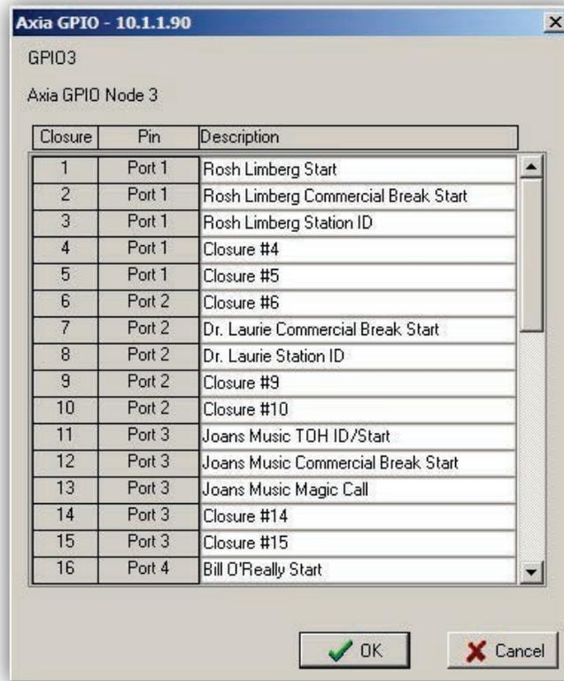
**Figure 4-19. Example of a Closure List**
