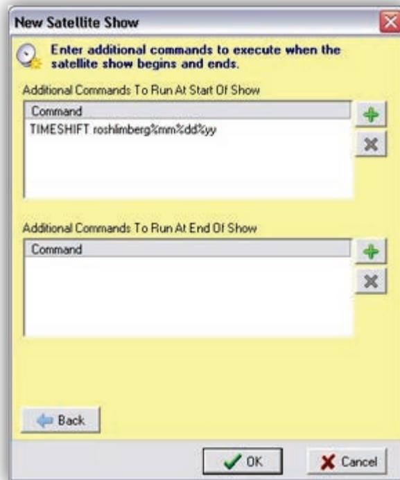
**Figure 8-11. Example of Using the TIMESHIFT Macro**
